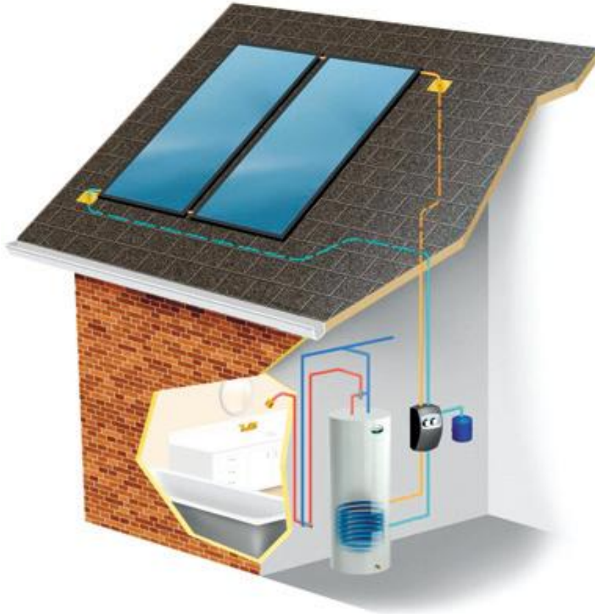
Solar DHW Solution
